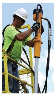
Easily accesible, quick release trigger, flat face quick couplings and vibration dampening, lightweight performance expedite post driving.
